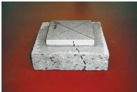
15 mm tile on concrete slab: Fracture of slab and tile at 37.800 N (average value)
