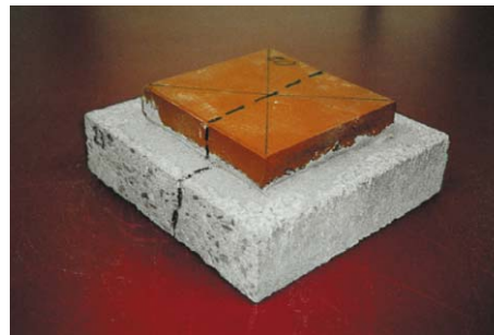
20 mm tile on concrete slab Fracture of slab and tile at 45.200 N (average value)
