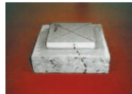
15 mm tile on concrete slab: Fracture of slab and tile at 37.800 N (average value)
