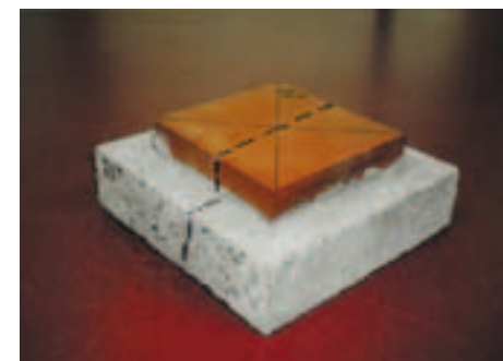
20 mm tile on concrete slab Fracture of slab and tile at 45.200 N (average value)
